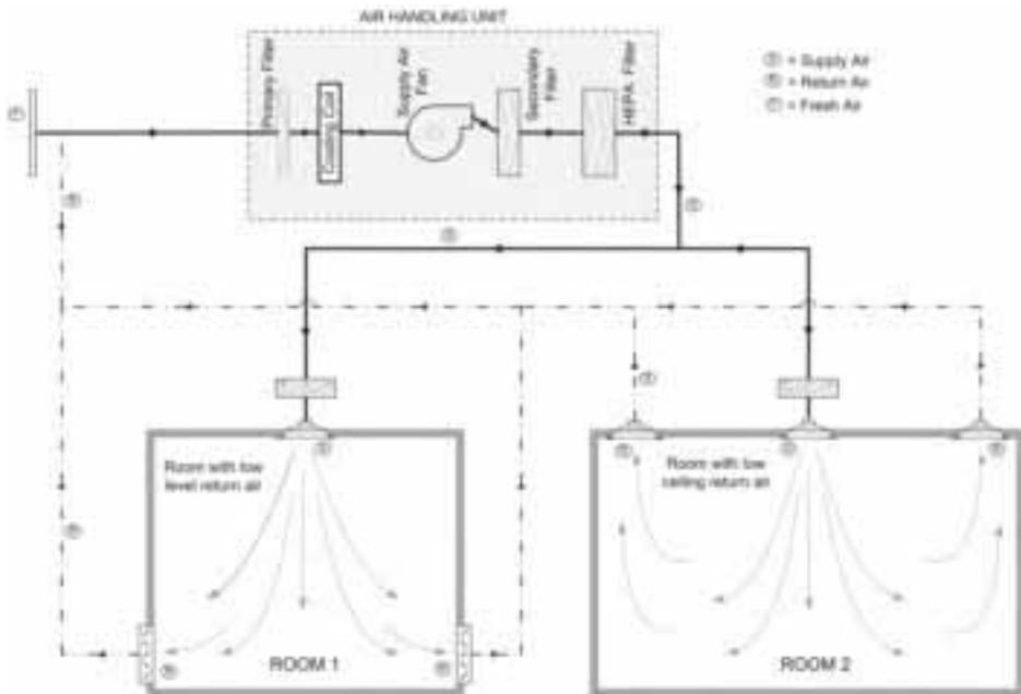
The airflow schematics of the two systems (Figures 22 and 23) indicate air-handling units with return air or recirculated air, having a percentage of fresh air added. Depending on product characteristics and dust loading it is sometimes preferable to fit filters on return air outlets or in return air ducting.
